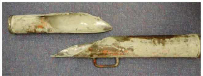
Photograph 2: Failed reducer—exploded view
