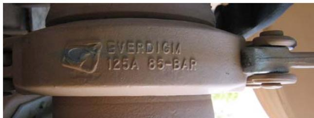
**Photograph 3:** An example of acceptable marking on pipe clamps.
