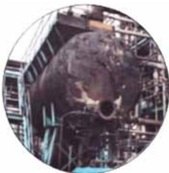
When heat was applied to the sludge (for about three hours) it generated a spontaneous, self-heating (exothermic) reaction that resulted in the ignition of the accumulated flammable gases present inside the vessel. (As it turned out, the assumed thermally stable tar was an unstable, tar-like liquid.)
