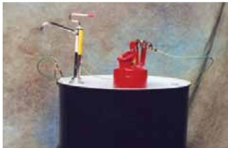
Figure 3. Drum pump with grounding clamps
