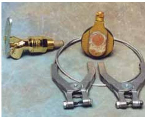
Figure 1. Self-closing faucet, safety bung and grounding clamps
