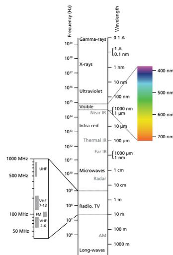
Figure 1. Radiation frequencies and wavelengths
